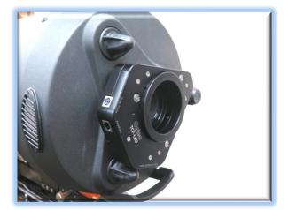
focuser drawtube, **you will need to move the focuser to the full OUT position**, or 112,000 steps. If you do not see the three setscrew hex heads because the drawtube is set too low, skip down to FocusLynx Software Setup below to configure and move the focuser drawtube OUT.
