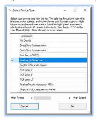
**High Torque**. With stepper motors, speed and torque typically work inversely. That is, higher speeds will usually result in lower torque. The TCF-Leo **High Torque** option can reliably handle payloads up to 10 kg or about 22 lbs.
