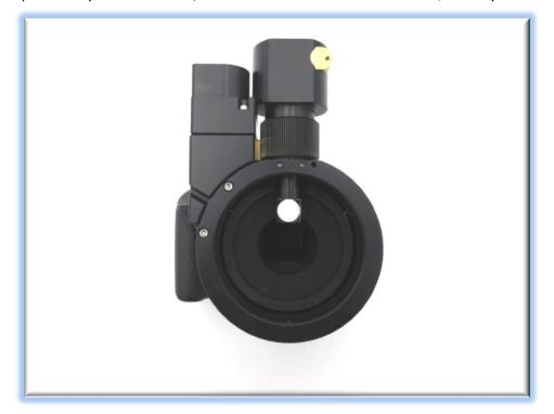
Rotate the OAG for best orientation and use the included 5/64" T-handle tool to tighten all three setscrews down tightly. Look directly down the front of the OAG. With the imaging camera shutter open you should be able to see the sensor. Orient the OAG such that the pick-off prism's lower edge is parallel to the long side of the imager sensor.
