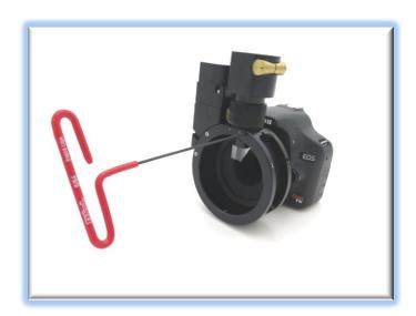
You may want to remove the AP2.7 male adapter from your OAG and attach it directly to your telescope before adding the Sagitta OAG. This will allow you to set the optimal orientation of the imaging package. With the best orientation, tighten down three oval point setscrews using the 5/64" T-handle. Securely tighten all screws to ensure a rigid, non-flexing imaging package.
