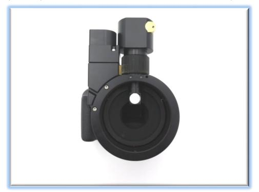
Rotate the OAG for best orientation and use the included 5/64" ball driver tool to tighten all three setscrews down tightly. Look directly down the front of the OAG. With the imaging camera shutter open you should be able to see the sensor. Orient the OAG such that the pick-off prism's lower edge is parallel to the long side of the imager sensor.
