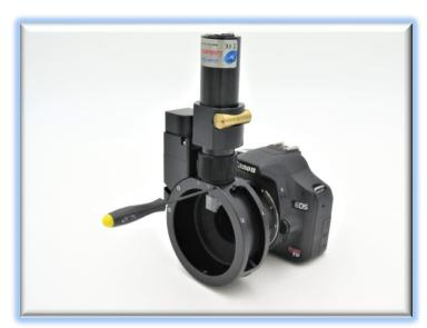
turn will lower the prism up closer to the sensor. Lower the prism until it is just above the imaging sensor as viewed from above.
