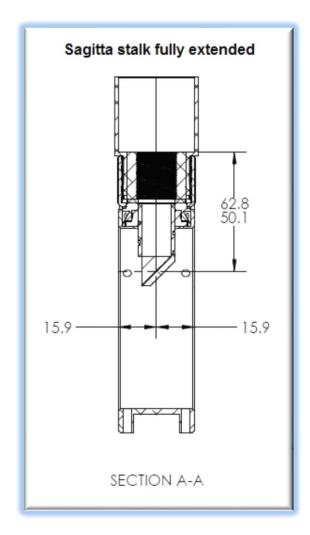
As an example, let's assume the pick-off stalk is fully extended and the focus mechanism is at the midpoint of travel. Then our guide camera OPL equates to 15.9mm (reference surface to prism center) plus 56.5mm (center of guide focus range [50.1mm to 62.8mm] to the seat of guide camera receiver) for a total guide camera OPL distance of 72.4mm.
