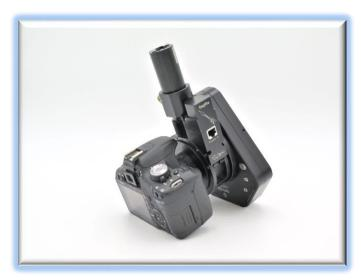
with the circular OPTEC-3000-S short dovetail adapters, you can set the optimal orientation of the imaging camera package. Rotate for the best orientation, then tighten down three oval point setscrews using the 5/64" ball driver. Securely tighten all screws to ensure a rigid, non-flexing imaging package.
