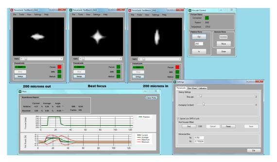
Designed as an ASCOM local server application with a pass-through methodology, FocusLock operates seamlessly and transparently to all other guide and imaging applications. Similar to Optec's Alt-Az Derotation Server software, the ASCOM shim is part of the magic behind FocusLock. As long as the telescope is guiding, the focus remains locked.
