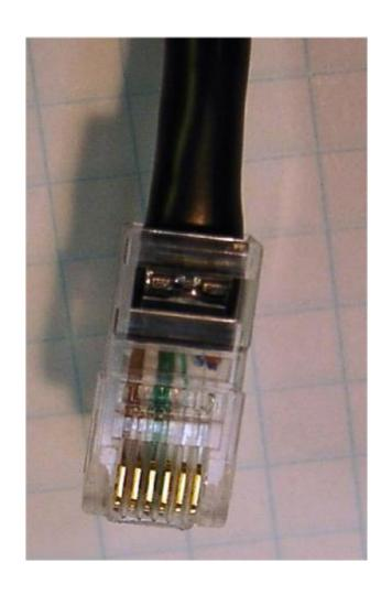
MOD8 (RJ45) and MOD6 (RJ12) crimped connectors using 4-wire telephone cable.
