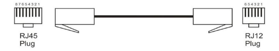
RJ12 Plug using Ethernet Cat5e cable. Pins 1 and 2 are not used.
