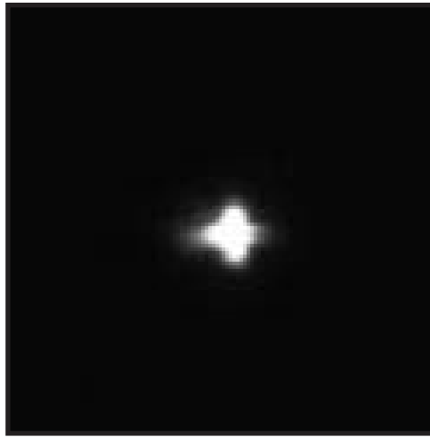
Image 3b - Guide star seen by guider camera (HFD = 5.2 px).
