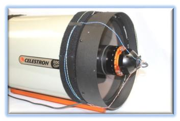
**Step 5**Wrap the Velcro cover strip around the circumference of the OTA over the wires adhering it to the Velcro cinch strap.
