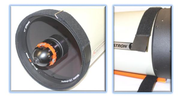
Install this bottom strap tightly around the OTA to provide a secure base for attaching the split-wire cable. Ensuring this base is tight will keep your wires taut.
