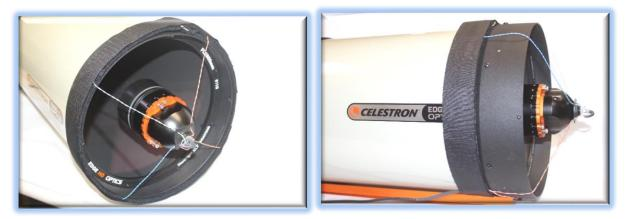
If you wish to fabricate your own split-wire kit from a standard Ethernet cable, contact <u>Optec Support</u> for a pdf showing the wiring layout lengths to fit either the Celestron EdgeHD C11 or C14 OTA.
