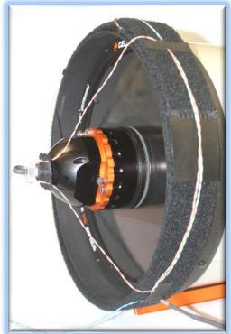
Smooth all four wire pairs against the base strap to prepare for the hooked cover strap.
