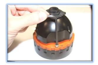
Test fit the FastFocus assembly onto the C-11 OTA confirming the alignment of the mark and alignment slot. Remove the entire assembly from the OTA. Remove the socket cap screws and the CTA adapter.
