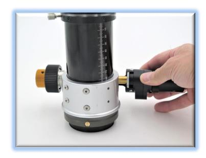
DirectSync ATX25 motor to the right and upward keeping the motor bracket parallel with the pinion assembly. Tighten the two M4 hex drive button head screws to secure the motor in place.
