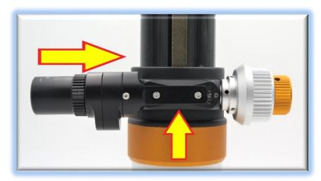
Test the mesh of the gears by engaging the motor. The coarse knob on the right side should not move when the motor is engaged.
