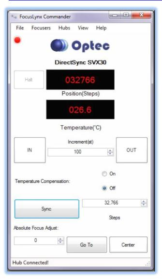
The ThirdLynx controller is an iFocuser3 type device. Because FocusLynx Commander is an ASCOM client, you will need ASCOM Platform 6.4 to configure the focuser. Visit the ASCOM webpages for the latest version.
