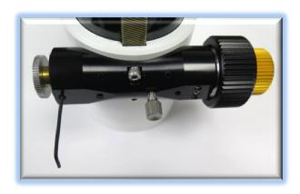
setscrew falls upon the flat section of the pinion shaft. Rotate the pinion shaft so the gear-hub setscrew can be seen through the access hole.
