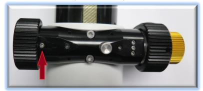
of the focuser. The coarse knob is fixed to the shaft with two metric hex set screws (also known as grub screws) that can only be accessed through a small threaded port on the main pinion block. You will use the 2mm hex head L-key to loosen these two setscrews. Loosen only, do not remove.
