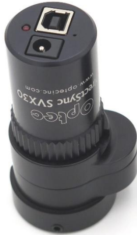
DirectSync SVX30 includes ThirdLynx control circuit
