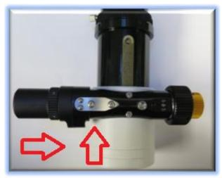
keeping the stainless tab parallel with the pinion assembly. You should still be able to see the setscrew holes through the stainless tab. Use two M4 hex drive pan head screws to hold the motor in place, the longer 6mm in the left and shorter 5mm in the right hole.
