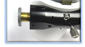
NOTE: Be sure to tighten gear setscrew tightly to avoid introducing backlash.
