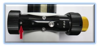
of the focuser. The coarse knob is fixed to the shaft with two metric hex set screws (also known as grub screws) that can only be accessed through a small threaded port on the main pinion block. You will use the 2mm hex head L-key to loosen these two setscrews. Loosen only, do not remove.
