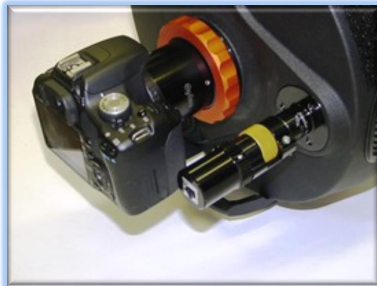
FocusLynx QuickSync motor with Feather Touch FTM Micro Pinion Retro-fit on a Celestron C11 HD.
