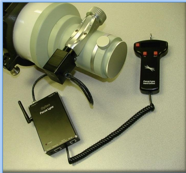
FocusLynx Controller Hub configured for MicroTouch motor. (Shown with FeatherTouch MPA/TRF pinion assembly on Takahashi TOA-130)
