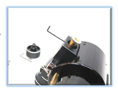
IMPORTANT: Tighten this setscrew securely to avoid introducing backlash from a loose fitting.
