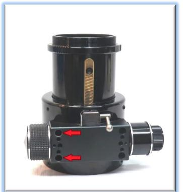
Examine the pinion block on the coarse side. Note the two largest holes (indicated in red below) have black socket cap screws holding the pinion block in place. We will remove these socket cap screws and replace with the stainless M4x0.6mm socket cap screws.
