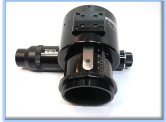
motor provides approximately 2.3 micron per step resolution and superior repeatability and load carrying capacity. A precision digital temperature sensor and electronic noise suppression circuitry are integrated into the DirectSync motor assembly. Connection to the FocusLynx control hub can be made using the included flat 8P8C or any other Cat-5e or higher network cable.
