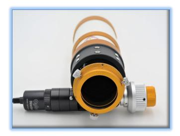
right-side coarse and fine focus knobs are left intact on the focuser while the DirectSync clutch mechanism offers easy engagement and disengagement of the stepper motor for manual focus.
