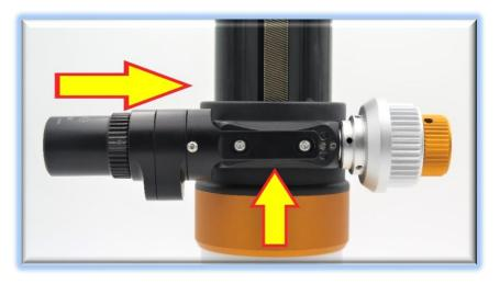
Test the mesh of the gears by engaging the motor. The coarse knob on the right side should not move when the motor is engaged. Disengage the motor (turn the motor cap counter-clockwise) and be sure the gears do not rub when the motor is disengaged. Adjust as necessary and re-tighten the M4 button head screws.
