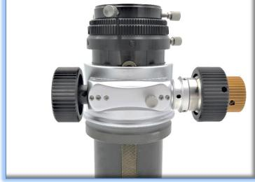
DirectSync AT25 motor provides approximately 1.4 micron per step resolution and superior repeatability and load carrying capacity. A precision digital temperature sensor and electronic noise suppression circuitry are integrated into the DirectSync motor assembly.
