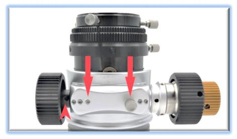
Next, remove the tension screw (if present) and the innermost setscrew on the coarse knob side of the pinion block.
