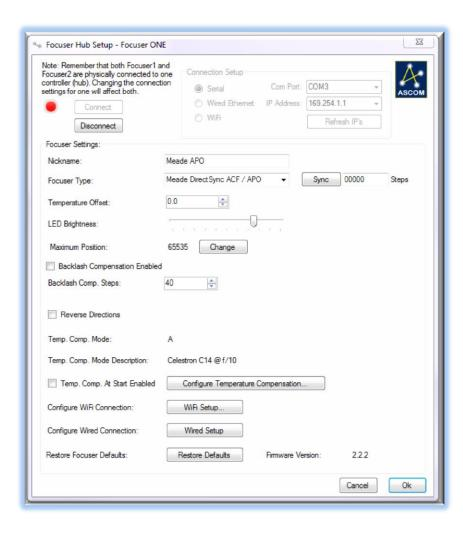
Type option. Your FocusLynx Hub firmware must be v1.0.6 or higher for this option to function properly. We recommend you turn on backlash compensation and set the number of steps to 60.
