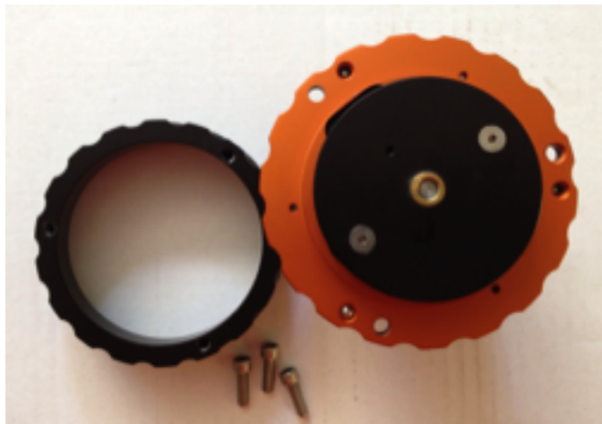
Picture of the housing – mounts on the corrector plate (well built)
