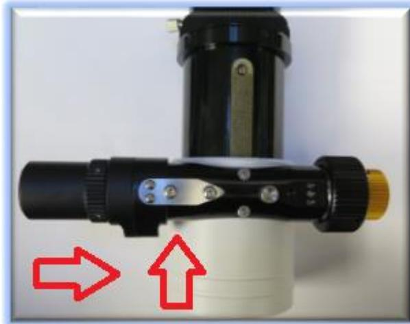
keeping the stainless tab parallel with the pinion assembly. You should still be able to see the setscrew holes through the stainless tab. Use two M4 hex drive pan head screws to hold the motor in place, the longer 6mm in the left and shorter 5mm in the right hole.
