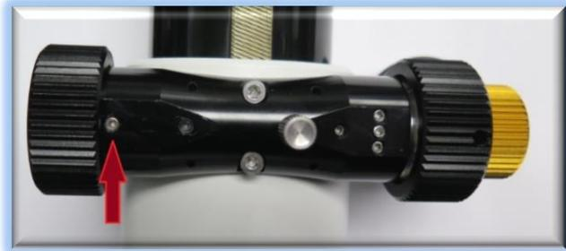
To access the knob setscrews, first use the 2mm hex key to remove the single setscrew indicated by the RED arrow below. Set the metric hex setscrew aside.
