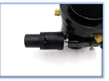
pin so that, when tightened, the end cap can no longer be rotated. Add the self-tapping M3 screw and tighten securely.
